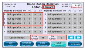
Set the current AGV route as route 1. When AGV passes through station 11, the current station will automatically switch to station 11 and perform a series of operations set in the previous step (empty operation will be automatically ski).
